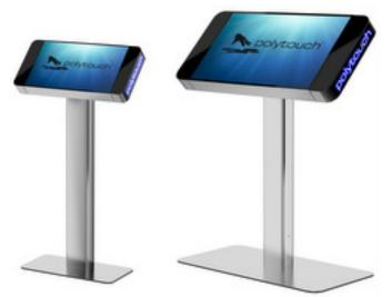
These Intel Core i7-3770S-driven units can detect 20 simultaneous touches at an ultra-fast 10 millisecond response time while rejecting palms resting on the screen. A neat trick to show off with at a show.
