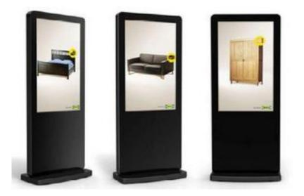
The new Medialine **Totem 4-series** are designed for 24/7 operation with DID panels of Samsung and AUO—and built with industrial metal housing and tempered glass.
