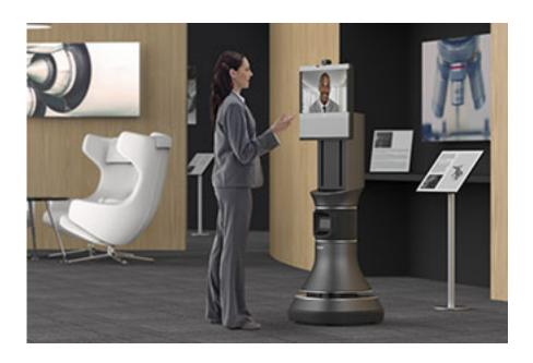
**Cisco's AV 500 iRobot** is a videoconferencing system driven by a robot. It's fully self-contained, battery powered and can move around a facility on its own,
