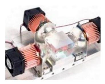
At InfoComm, Wavien, Inc. showed its **Recycling Light Technology (RLT)** that increases brightness of LEDs for small target illumination in the digital projection.
