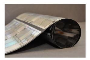
PowerFilm gave a live demonstration of the world's first and only backplane array technology for a flexible display (made using a full roll to roll process integrated with a front plane driver to create the full working display). A backplane driver is an array of transistors that turns individual pixels on a display on and off, according to instructions from a computer.
