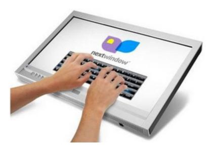
EIZO is using the NextWindow 1900 Desktop Touch in its new tilt-able FlexScan computer monitors. Users can interact with the 1900 series while wearing gloves, as in medical environments. It also provides traditional touch functions such as point, click, drag and drop, as well as multitouch functions like pan, pinch, double-tap and scroll.
