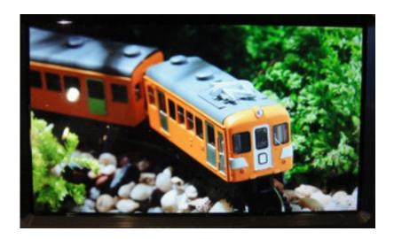
What HAST man wrought? Ortus creates a Hyper Amorphous Silicon TFT (HAST) screen. Shown at Tokyo's Embedded Systems Expo, the latest 4.8" LCD screen from Ortus shows 2D images at the 458 pixels per inch rate and shows 3D images at 229 pixels per inch. This rate of pixels per inch will be able to show full HD resolution images with a final resolution of 1920 x 1080 pixels.
