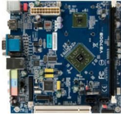
It combines a 1GHz C7 processor with as the VX900 into a unfied media system processor handling HD video, audio and HDMI support in a compact power-efficient package measuring 17 x 17cm.
