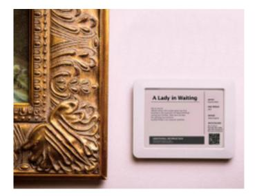
The AMLABEL Digital Gallery Display in USA is an editable, real-time in-gallery digital label developed on electronic paper to replace existing gallery cards.
